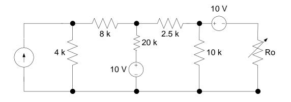
(a) source transform: Find open circuit voltage.
